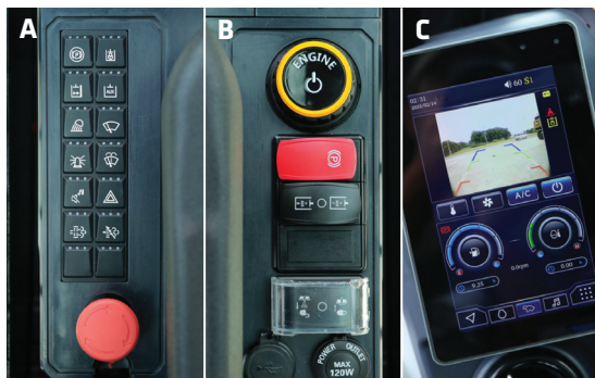
[A] Multifunctional control panel for easy and convenient operation. [B] One-click startup; one-click unlock. [C] 7" LCD display.
