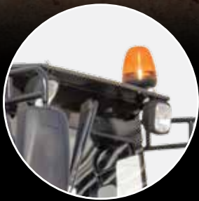
1. FRONT/REAR CAB LIGHTS AND BEACON
