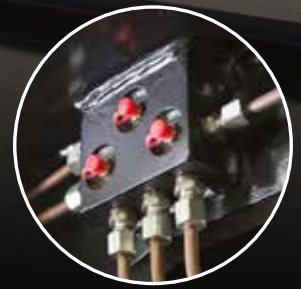
4. CENTRALIZED GREASING POINTS FOR THE MAST AND STEERING PIVOT PIN
