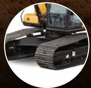
8. LONG, HEAVY-DUTY UNDERCARRIAGE FOR STABILITY AND DURABILITY
