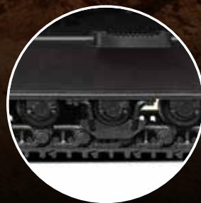
7. SEGMENTED TRACK GUARDS TO KEEP TRACK IN PLACE AND REDUCE WEAR
