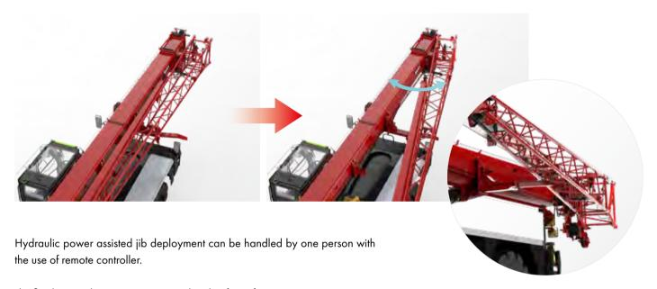
The fly jib gives the crane an extra tip height of 176 feet.
