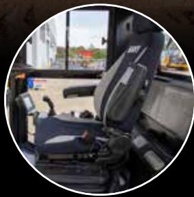
6. AIR RIDE HEATED SEAT (SSR120C-8 & SSR120HT CAB MODELS)
