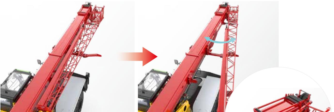
Hydraulic power assisted jib deployment can be handled by one person with the use of remote controller.
