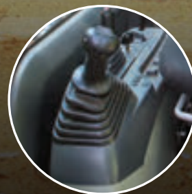
4. HYDRAULIC PILOT CONTROLS WITH PATTERN-CHANGE SELECTOR
