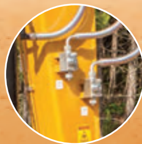
3. 1- AND 2-WAY MAIN AUXILIARY AND 2-WAY ROTATE AUXILIARY HYDRAULIC PIPING
