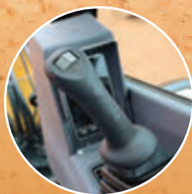
5. HYDRAULIC PILOT CONTROLS WITH PATTERN-CHANGE SELECTOR
