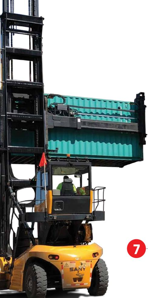
An abundance of thought has gone into machine serviceability. There are no special tools or computers needed to trouble shoot issues. The operator can view all codes through the monitor located near the right console. Daily checks can be completed quickly with the convenient layout of the visual check points for the engine oil, transmission fluid, and hydraulic fluid.
