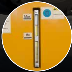
6. SEPARATE BRAKE AND HYDRAULIC TANKS
