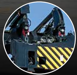
8. SPREADERS ARE CHAIN HUNG TO THE GANTRY
